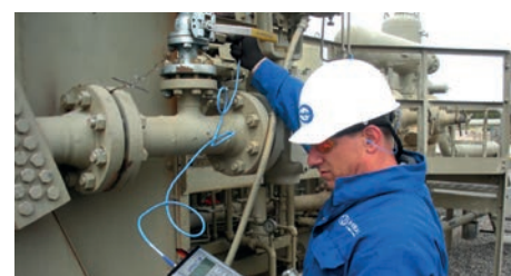
Inspection of leaking valve with VPAC II™
